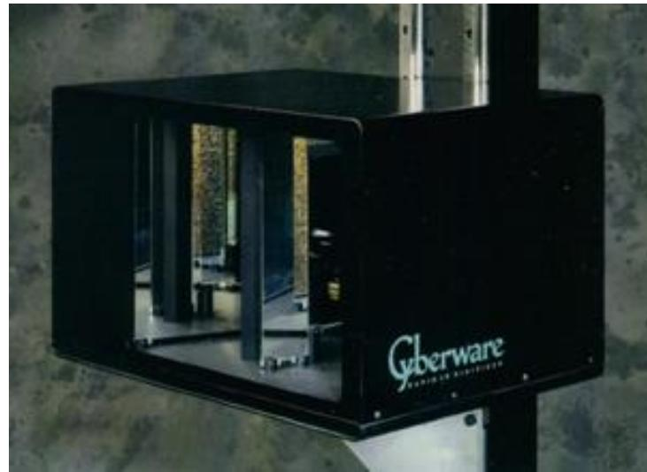
Slika 6. Laserski skener (Cyberware, Inc. Monterey, Kalifornija, SAD).
