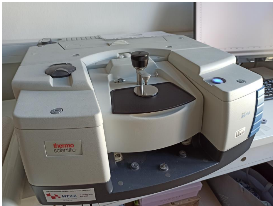
Slika 9. Infracrveni spektrometar Nicolet iS50 (Thermo Fisher Scientific, Waltham, MA, SAD).
