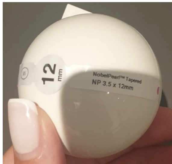
Figure 1. NobelPearl Zirconia Material in Raw Form for Dental Implant Fabrication Courtesy of Professor Carek
