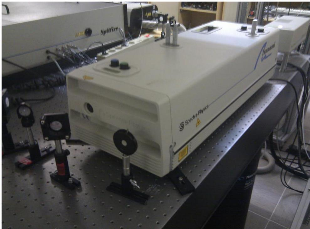
Slika 18. Femtosekundni laser (Millenia, Spectra Physics, SAD).
