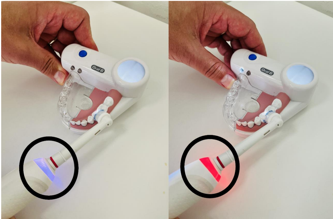
Figure 5: Smart pressure sensor changing colour depending on pressure; blue = normal pressure; red = excessive pressure.
