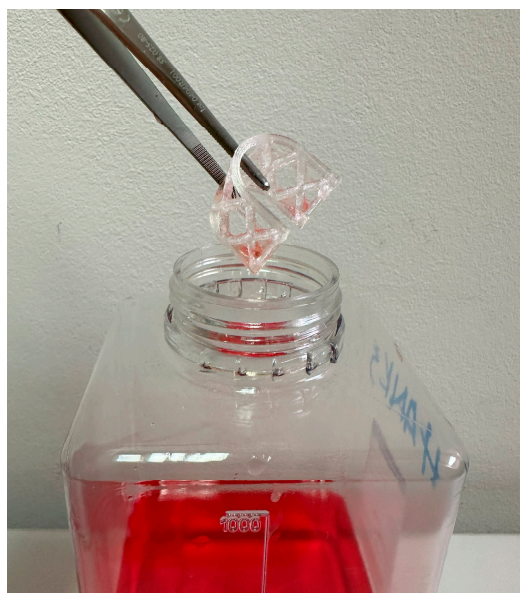
Figure 7. Biodegradable augmentation scaffold removed from Hank's balanced salt solution using sterile stainless steel forceps.
