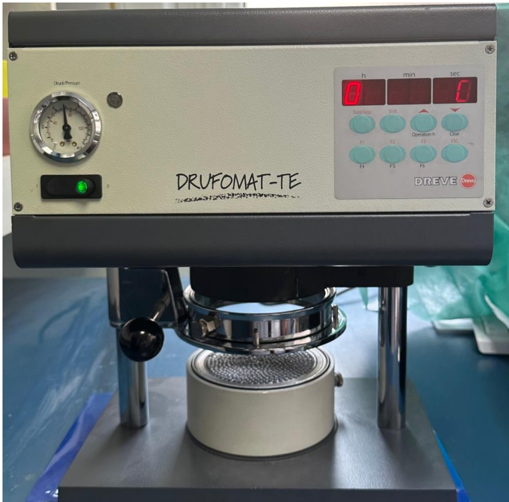
Figure 3. Dreve Druformat-Te mouthguard manufacturing device
