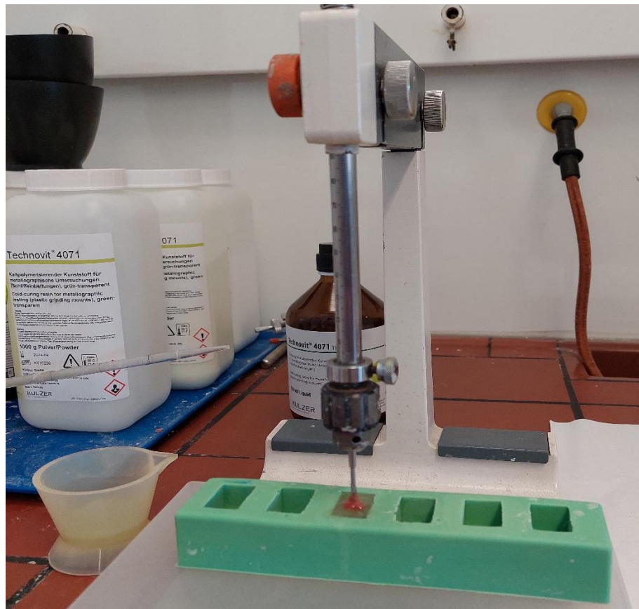
Figure 13. Sample preparation with autopolymerising acrylate.
