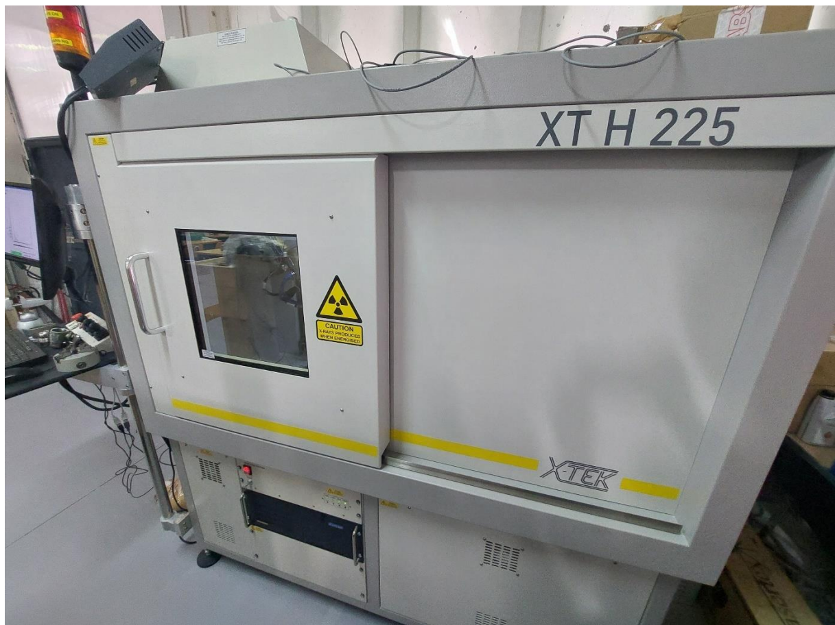
Figure 20. Micro-CT device used for remineralization imaging.
