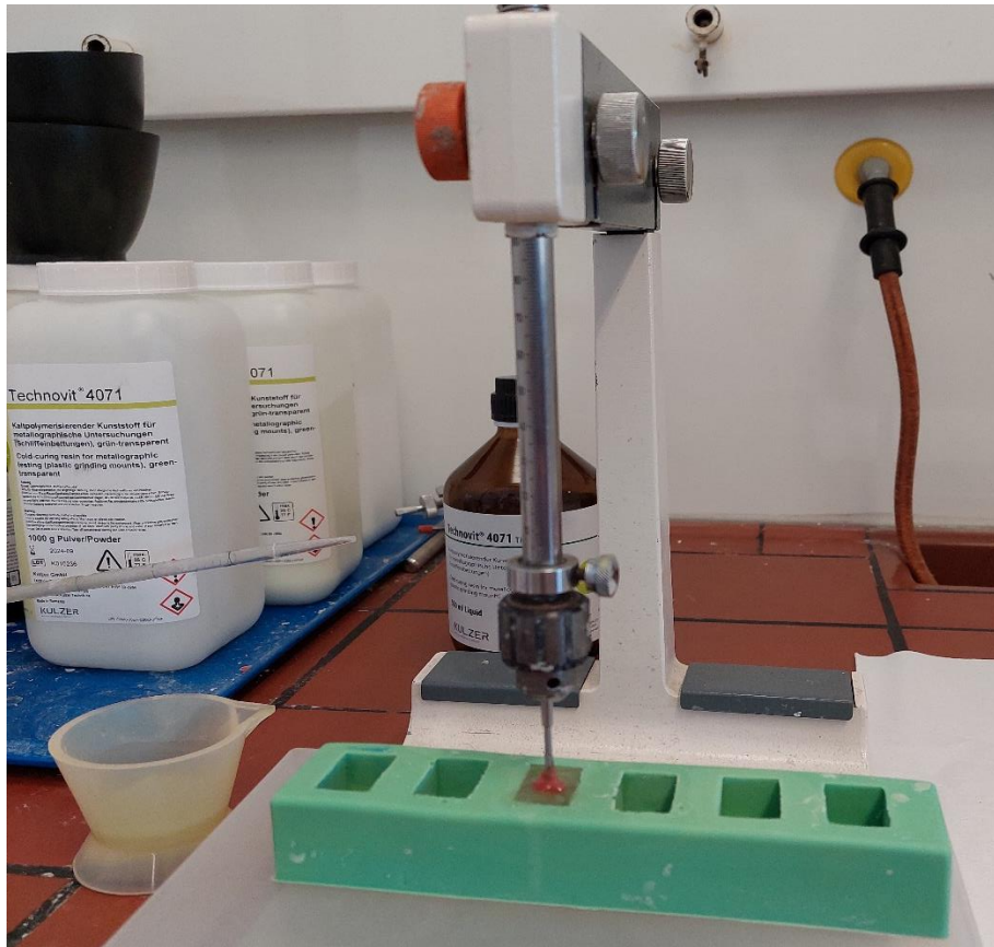
Figure 13. Sample preparation with autopolymerising acrylate.
