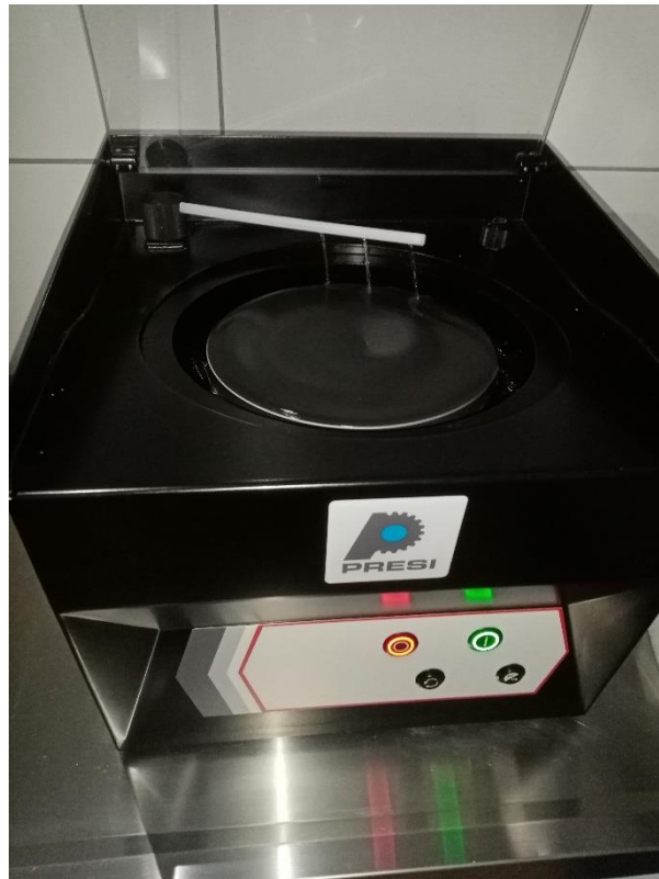
Figure 8. Polishing device used in the study.
