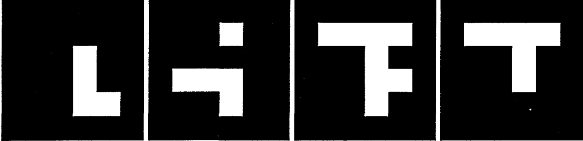
Figure 2: The four planes of a near-optimal 3-D binary structuring element obtained by means of GA. The SE size is 4 \times 4 \times 4 .
