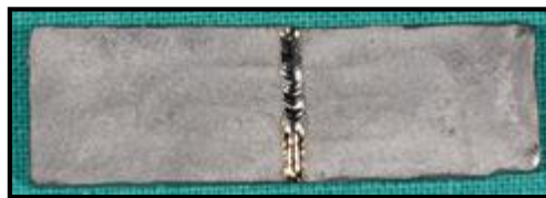
Fig. 3. Face of weld of laser welded casting; Sample 3
