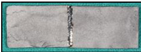
Fig. 2. Face of weld of laser welded casting; Sample 2
