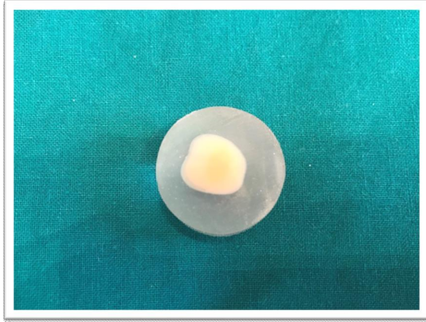
Figure 9. An artificial tooth immersed in a colorless cold-polymerized acrylics
