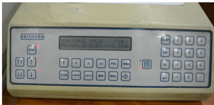
Figure 11. The force required to debond the brackets was recorded in Newton.
