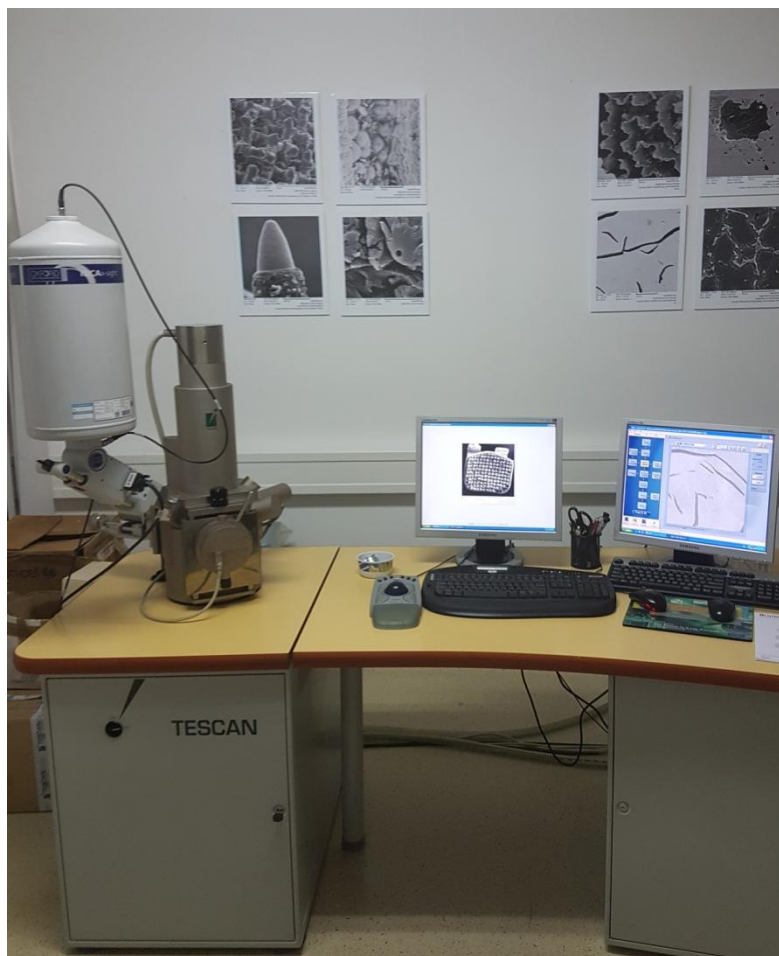
Figure 12. Scanning Electron Microscope - Tescan Vega.
