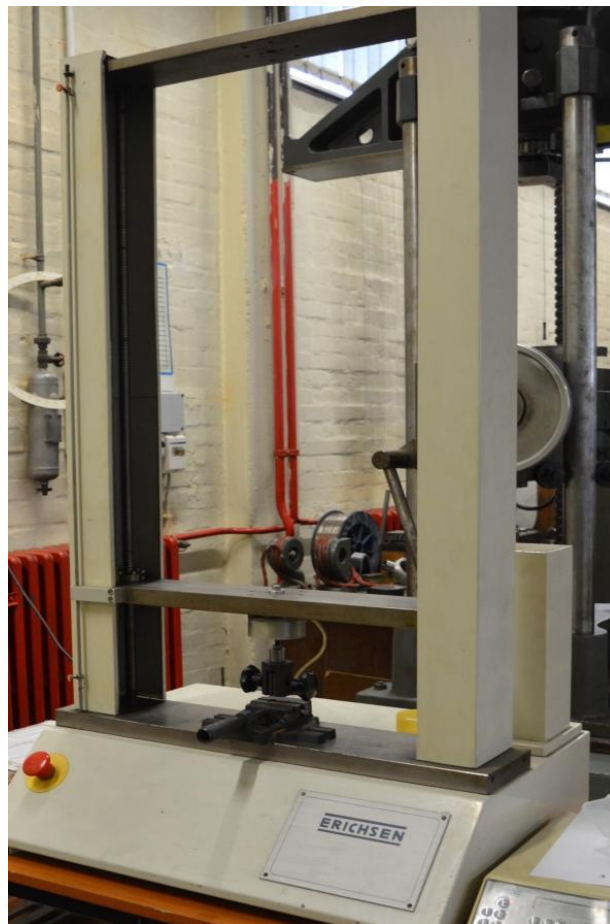
Figure 9. Universal Testing Machine - Erichsen 0-2000 N.
