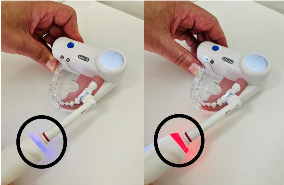
**Figure 5:** Smart pressure sensor changing colour depending on pressure; blue = normal pressure; red = excessive pressure.
