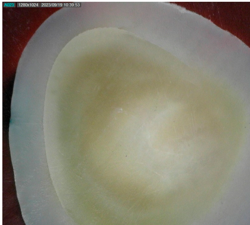
Figure 2. Image of a specimen with adhesion fracture under a Dino-Lite digital microscope.
