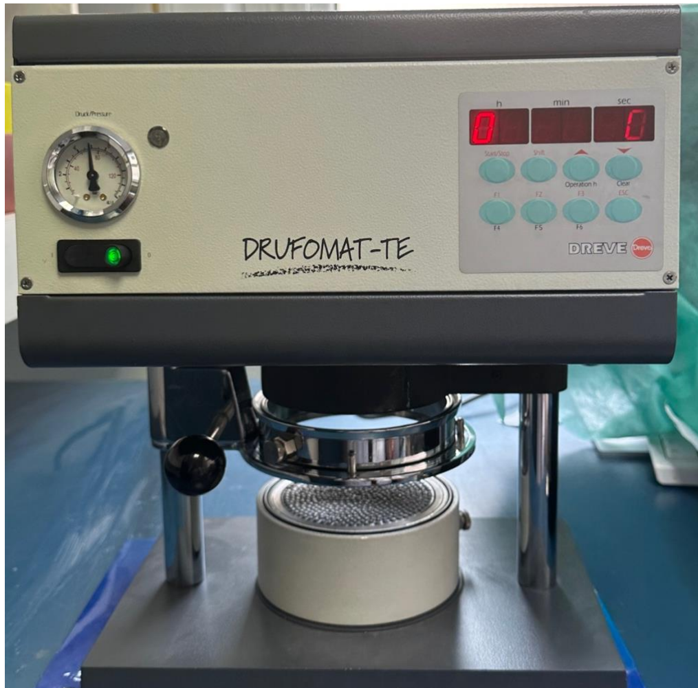
Figure 3. Dreve Druformat-Te mouthguard manufacturing device
