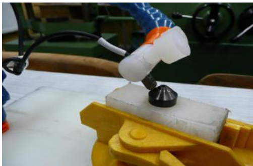
Fig. 1: Workstation for pitting phenomenon examination [left]; schema of the examined cone [right]
