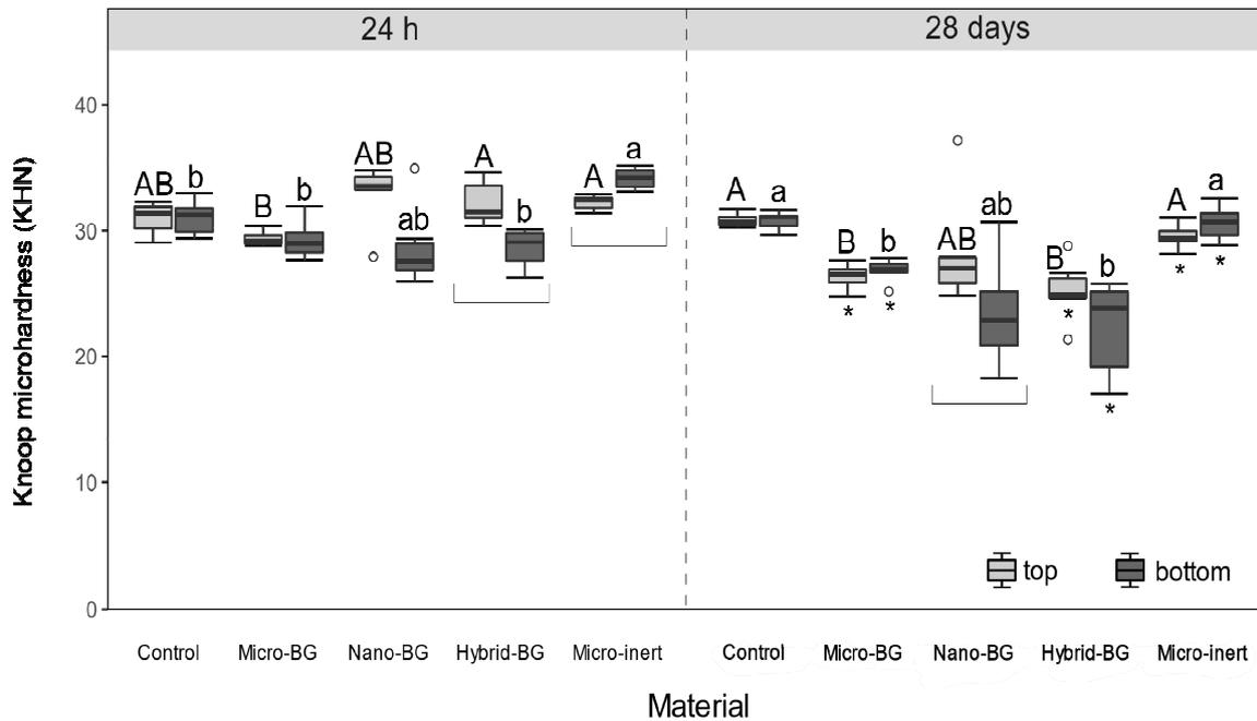
**Figure 3.** Knoop microhardness measured after 24 h and 28 days. Within each measuring time, same uppercase letters indicate statistically homogeneous groups for top surfaces, while same lowercase letters indicate statistically homogeneous groups for bottom surfaces. Asterisks (\*) indicate significant differences between measuring times, within each material/surface combination. Square brackets indicate significant differences between the top and bottom surfaces.
