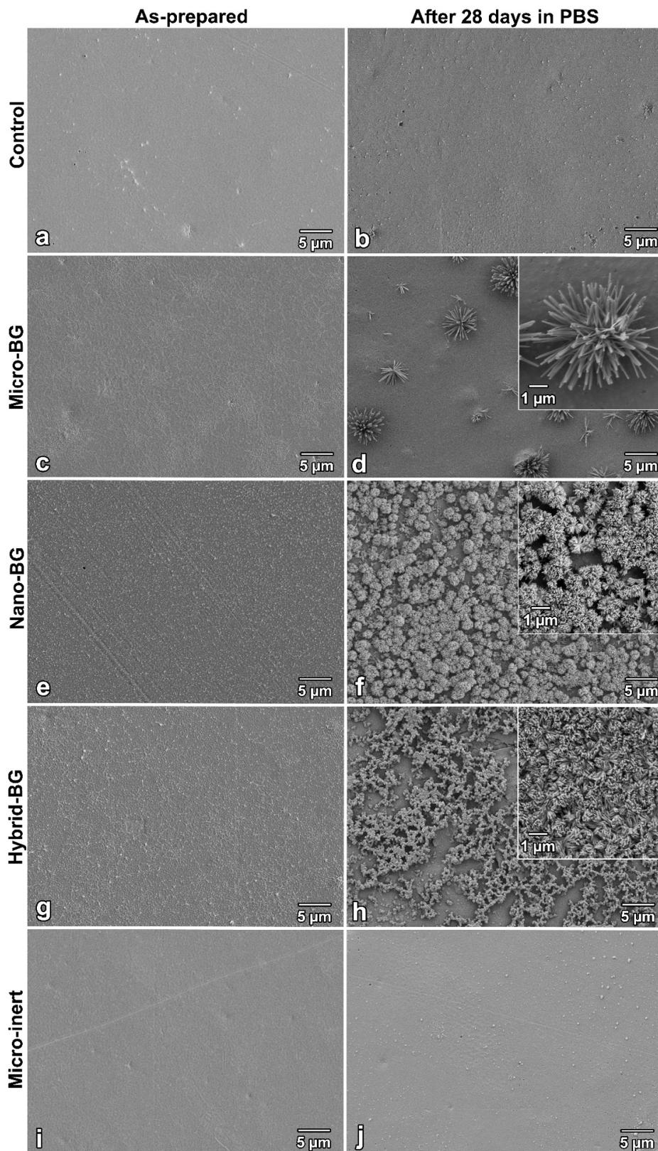
**Figure 4.** Scanning electron microscopy images of specimen surfaces immediately after preparation and after 28 days of storage at 37 °C in phosphate-buffered saline (PBS) for the control (a,b), micro-BG (c,d), nano-BG (e,f), hybrid-BG (g,h), and micro-inert composites (i,j). Insets show higher magnification of crystals formed on specimen surfaces.
