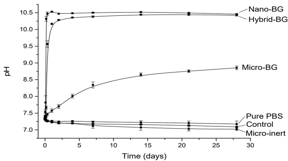
Figure 1. pH (mean  $\pm$  standard deviation) as a function of immersion time.
