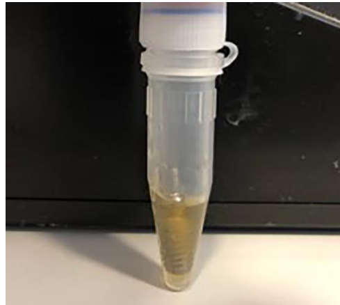
Figure 7. Implant assemblies immersed in a solution contaminated with S. aureus and C. albicans , in Eppendorf tubes.
