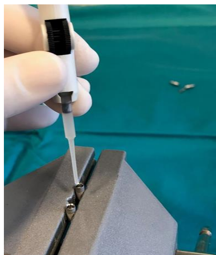
Figure 3. GapSeal gel application.
