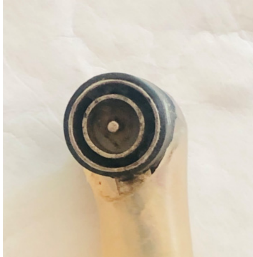
Figure 1. Intraoral probe consisting of 3 concentric aluminium alloy electrodes.
