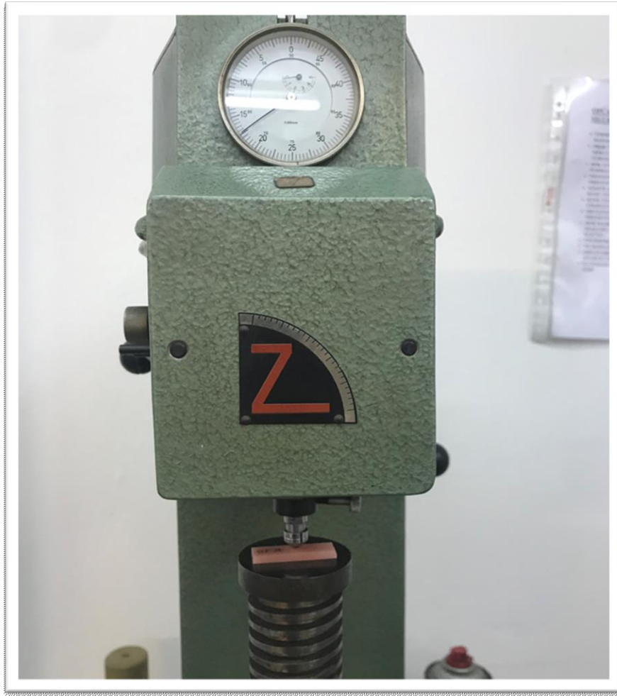
Figure 4. Zwick apparatus used for surface hardness testing
