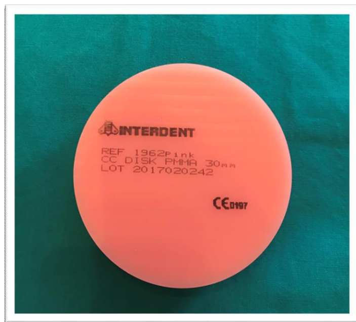
Figure 8. Material for a milled denture base – Interdent CC disc PMMA
