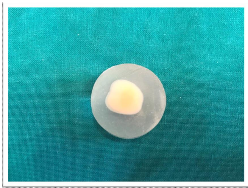
Figure 9. An artificial tooth immersed in a colorless cold-polymerized acrylics
