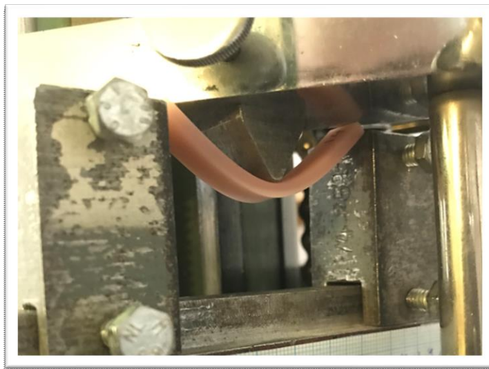
Figure 2. An undamaged CAD/CAM specimen (IvoBase CAD) with loading within the end limits of the possible movement of the penetrant
