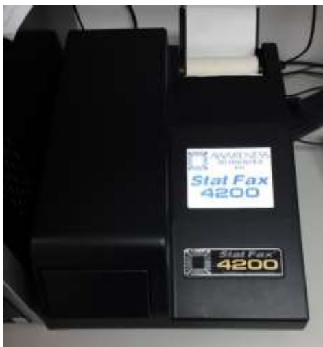
Slika 14. Fotometar čitač ( Awareness Technologies Stat Fax 4200 Microplate Reader, GMI, Ramsey, USA ).
