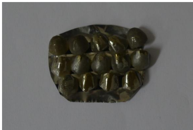
Figure 14. The samples after sputtering with palladium/gold coater.
