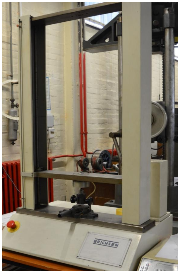
Figure 9. Universal Testing Machine - Erichsen 0-2000 N.
