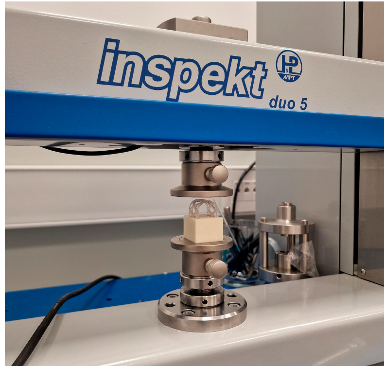
Figure 5. Occlusal compression test on Universal testing machine Inspekt table 50 kN.
