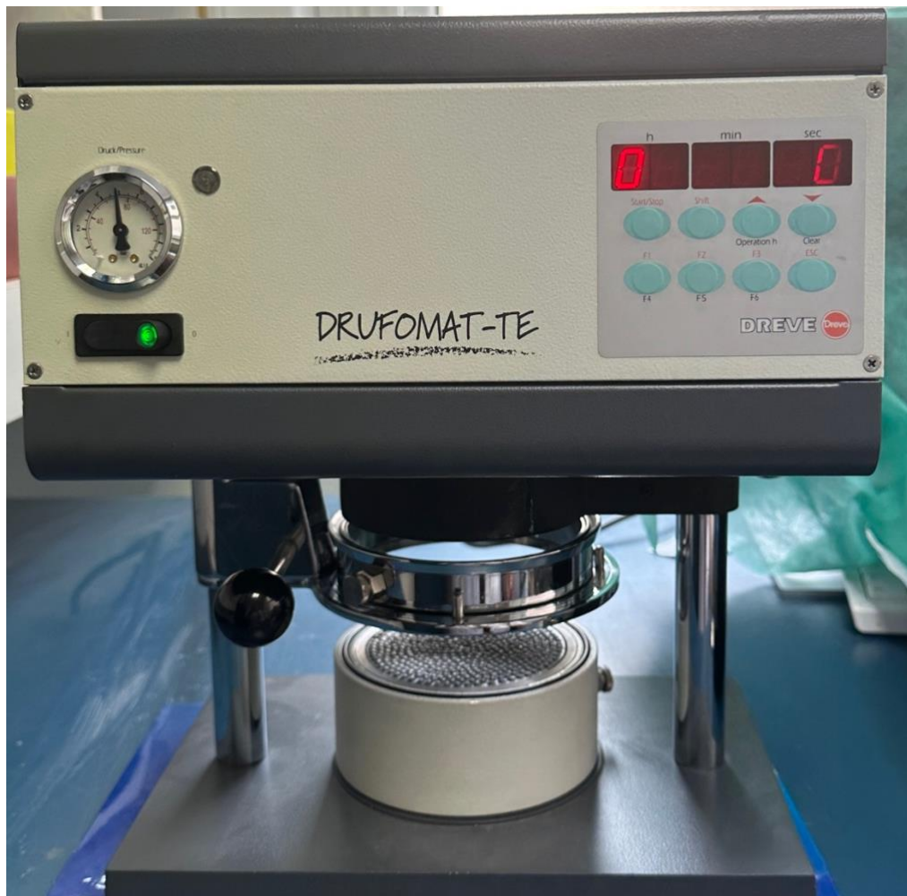
Figure 3. Dreve Druformat-Te mouthguard manufacturing device
