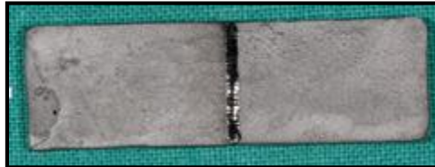
Fig. 1. Face of weld of laser welded casting; Sample 1
