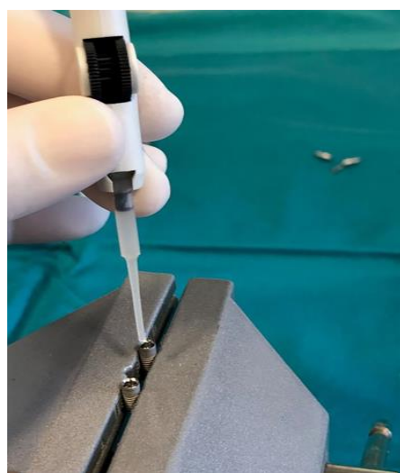
Figure 3. GapSeal gel application.
