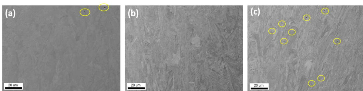
Figure 3. Microstructure of specimens: (a) Sysma MySint100, (b) EOS M100, (c) 3D Systems DMP Dental 100. Yellow circles mark porosities.
