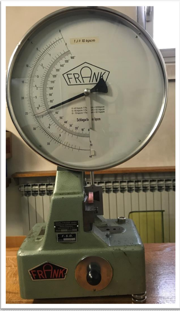
Figure 5. Charpy's bar used for an impact strength testing
